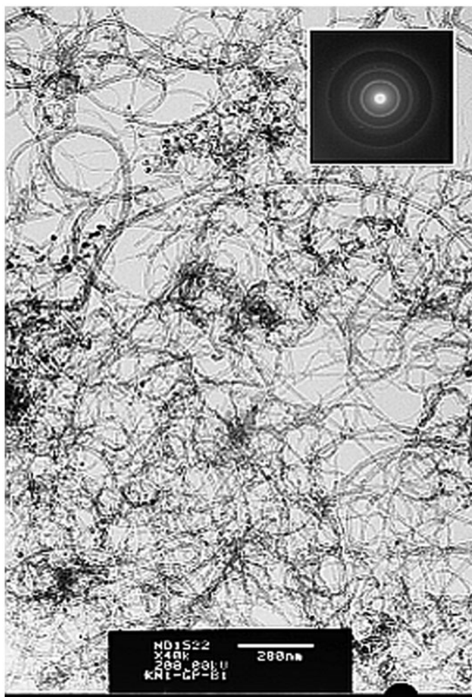
Figure 1. TEM micrographs of CNT in transmission regime and SAED regime (insert in the right corner).
